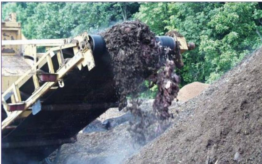
After grinding, the product will be placed on an 18 to 24-inch-thick bed of carbon material. This product forms the core of the windrow. A cap (again made of the carbon material) will be placed on top of the core at a thickness of 18 to 24 inches. The typical finished windrow height is six to eight feet tall and 12 to 16 feet in width.
